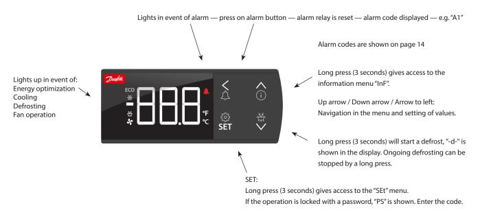
Shows the setting for a chosen parameter / saves a changed setting. Short press gives access to entering of the thermostat's cut-out limit.
