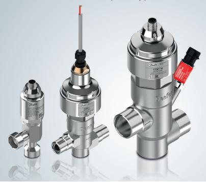
The CCMT is a highly reliable electric pressure regulating valve optimized for transcritical CO<sub>2</sub> refrigeration. The valve has versatile applications in the transcritical system. The valve is capable of high pressure gas cooler control (transcritical). The CCMT can be used as gas by-pass valve (medium pressure control). If desired, the valve can also be used as a normal expansion valve for evaporators.
