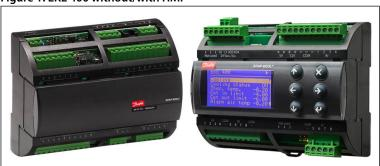
For industrial refrigeration applications the Danfoss EKE 400 can control the operation of the valves and the fans for evaporators to achieve optimal cooling mode and defrost sequence for an efficient, safe and trouble-free operation of the evaporators, complying with IIAR(3) safety recommendations for hot gas defrost.
