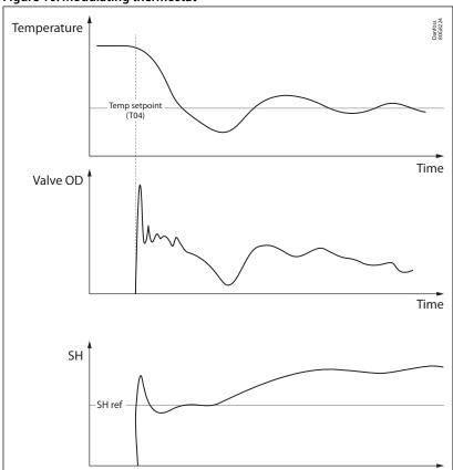
Figure 10: Modulating thermostat
