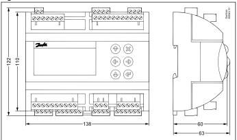
For DIN rail mounting only (IP 20)
