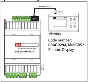
When setting up EKE 1A to operate ETS 6, ETS, KVS, ETS Colibri®, KVS Colibri®, CTR, CCMT valves, but controlled from EKE 400,
